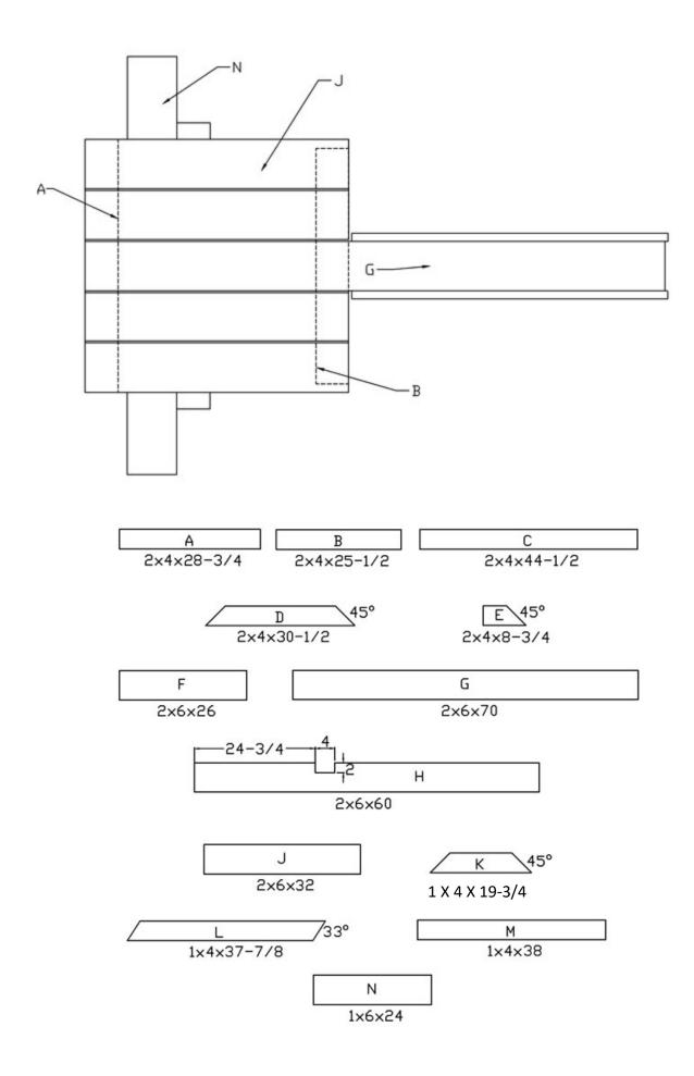
Basic Bench Cutting Diagram, 8' boards, without transmitter/parts holder.
