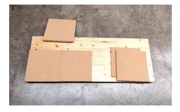
Finally, I cut the remaining two panels in half and completed the board. Take care to align the edges so there are no gaps:
