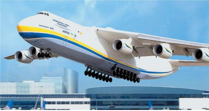
Only one An-225 has ever been completed. It first flew on December 21<sup>st</sup>, 1988, and was designed primarily to transport orbiters for the Soviet space program. In addition to being the heaviest aircraft ever built, it also has the largest wingspan of any aircraft currently in operation: 290 feet.
