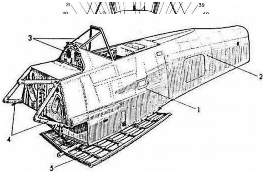
Let's take a look at the FW-190's construction. The basic fuselage structure consists of 2 parts the forward (1) and aft (2). The drawing also shows a large removal panel on the underside (5) which allows access to the self sealing fuel tanks. Dural was used extensively and results in a much "tougher" airframe. The modern equivalent to Dural is the 2000 series of aluminum with the aluminum being alloyed with copper.
