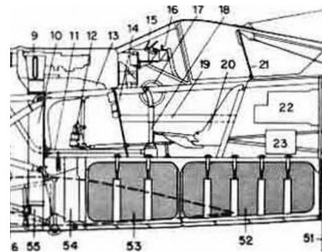
Presumably this gave the pilot a higher G tolerance similar to the semi-reclined pilot seat in the F-16. The picture also shows the 2 large self sealing fuel bladders (52 & 53) located below the cockpit floor. Allied fighter pilots sat in a normal position which was less tiring.
