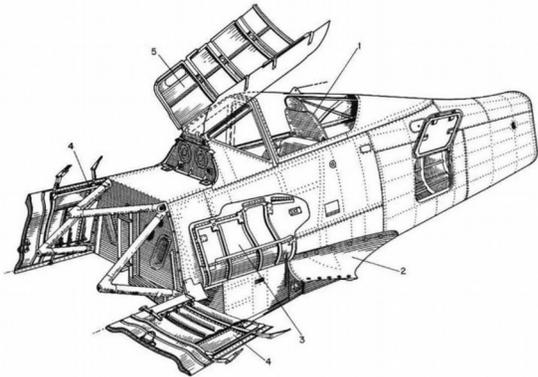
There were large access panels in many areas of the aircraft allowing for ease of maintenance to get the aircraft back in the fight as quickly as possible.
