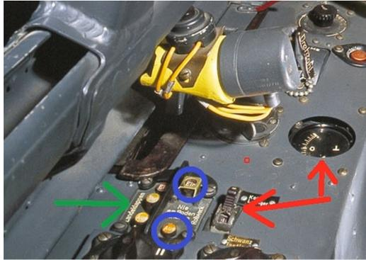
For engine and propeller control the FW-190 had a device called Kommandogerat which managed all factors of the engine. All the pilot had to do for different flight regimes was move the throttle to different boost settings and the device
