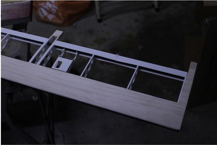
So how does this relate to the spar in the glider wing? I believe it was an attempt by the designer to maximize wing performance by maintaining a smooth airfoil contour all along the wing chord. There is no spar bump to cross. Instead the covering follows the rib contour at the ribs and between the ribs it smoothly changes airfoil contour to a thinner airfoil section midway between the ribs and then smoothly changes back to the rib profile.
