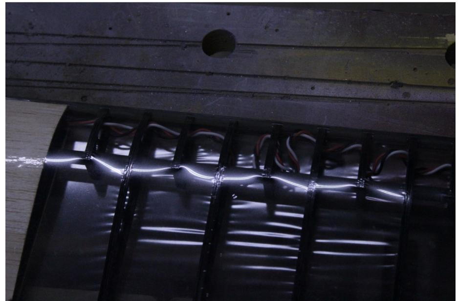
The replacement wing has leading edge sheeting (balsa) back to the spar. The much stiffer sheeting does not sag between the ribs. However, behind the spar the covering still does not maintain contour and there is a subtle “kink”. This kink could lead to flow separation and stall or simply degrade the wing’s performance.
