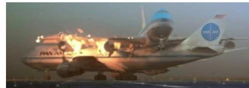
The KLM plane remained briefly airborne, but the impact had sheared off the outer left engine, caused significant amounts of shredded materials to be ingested by the inner left engine, and damaged the wings. The plane immediately went into a stall, rolled sharply, and hit the ground approximately 500 ft past the collision, sliding down the runway for a further 1,000 ft in a ball of fire.
