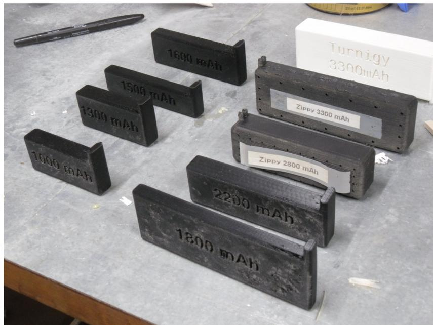
I've found that having battery simulators are very helpful in trying out combinations of batteries without the expense and wasted time of buying them. I 3D print mine because I have a 3D printer but if you don't you can try cutting simulators out of foam or wood. Label them with capacity and manufacturer and store them where you can find them later. On my simulators I include a "nub" to represent the wires exiting the battery.
