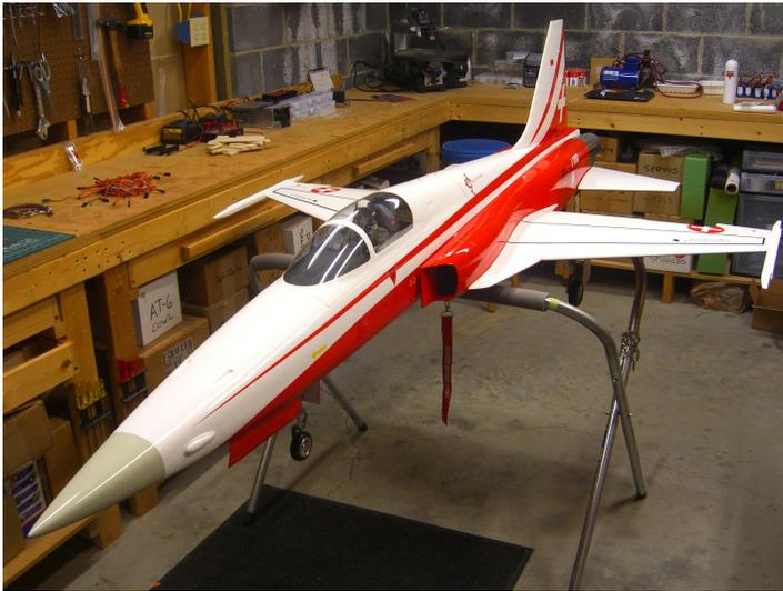
which should result in a take-off weight slightly north of 40 pounds with a gallon and a half of Jet A on board.
