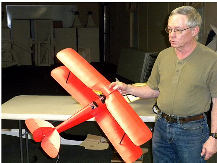
shrinks with heat. The rest of the setup is a 10Amp ESC and 8x3.8prop on an unknown kv motor. This 3 channel plane "flies like a pussy cat" and gives him about 20min of flying with his setup.
