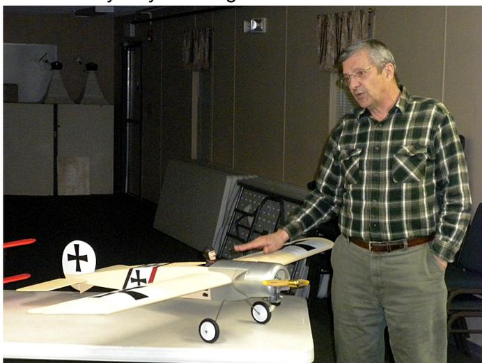
Eindecker kit covered with Solartex fabric and with an OS52 4 stroke motor. Some decals were painted on with white spray paint and others were made by a friend of Gene Waters in Oak Ridge. .
