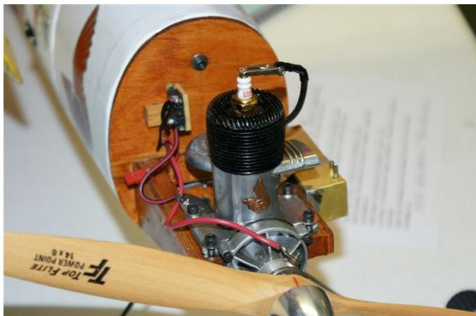
This is the Ohlsson .60 ignition engine used to power the Sailplane. It was maybe the best in its class.. It used points, coil and condenser plus a battery to generate a spark, and there was no throttle; it was fullbore loud all the time.
