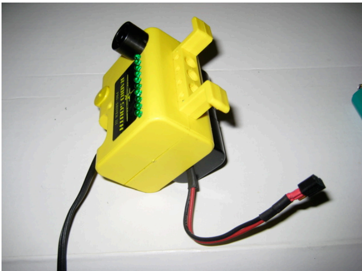
photo 4; Completed unit showing new charge lead.
