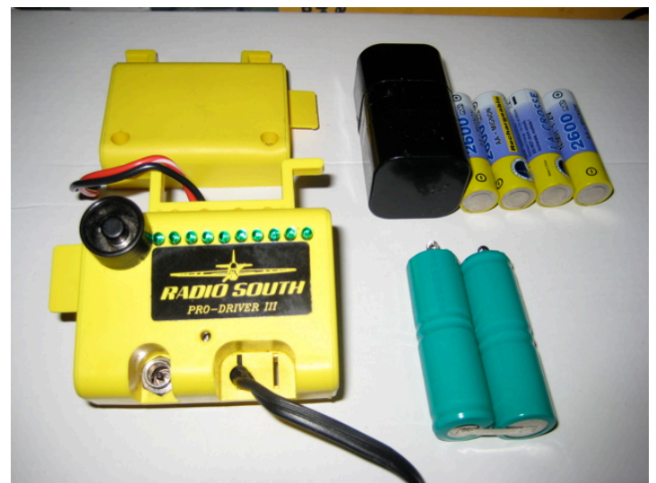
photo 1; Radio South Pro-Driver III, stock cells (green) and planned replacement cells (2600 mAh cells, upper right) along with the black Futaba battery box from days-of-old.
