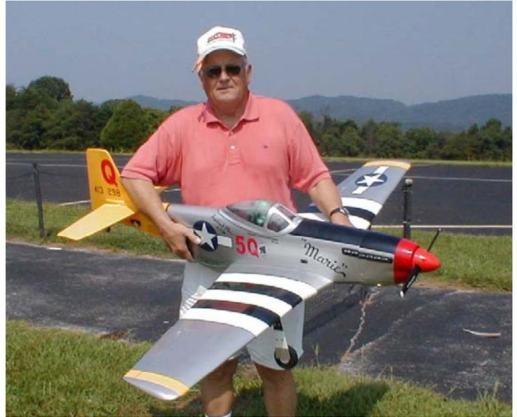
Charles Wilson also is sporting a new one. His is one of the P-51 ARFs sold by RaidenTech. The fuse is fiberglass and the wings and tail structure is built up. The model is a good sized one with a wingspan of ~ 66 inches.
