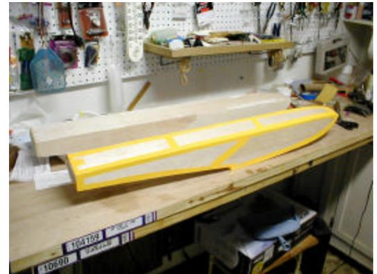
the finish. Whether or not to fiberglass. On the prototype, they just covered them with Monocote, doubling up on the seams, and said they were happy with the results, so I decided to try that also. The second picture shows the seams covered with Ultracote on one of the units. I will cover over the whole unit now with Ultracote. I will report on the progress in the April issue.
