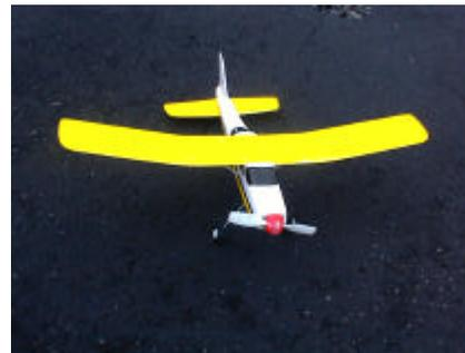
The wingspan is about 10 inches. It is powered by one small nicad cell which is charged by connecting a 2 cell AA battery pack to it for ~ 2 minutes. John would stand in the middle of the runway and hand launch it and it would circle around his head
